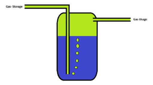
The safest way is to make two of these systems. One close to the digester, and one close to the end-usage. (cookingstove)
